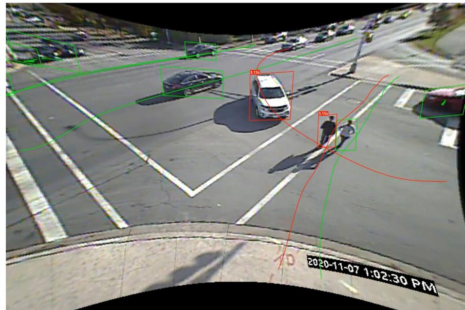
Pedestrian North Left-Hook:  $T_2 = 1.6s$ , vehicle speed 20 km/h
