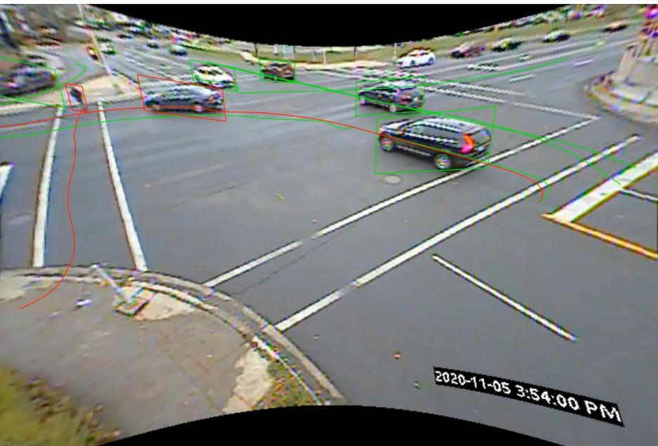
Pedestrian West Left-Hook:  $T_2 = 2.6s$ , vehicle speed 14 km/h
