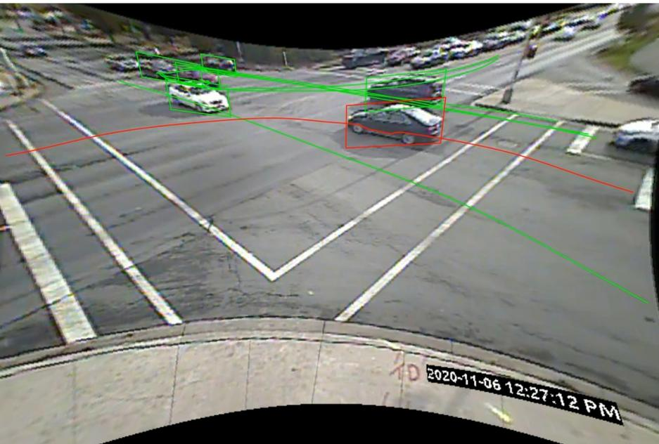
East-left vs West-through: PET = 1.6s, vehicle speed: 56 km/h
