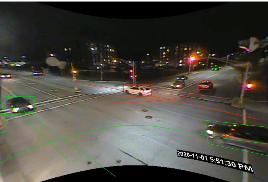
West-Left vs East-Through: PET = 1.5s, vehicle speed = 65 km/h
