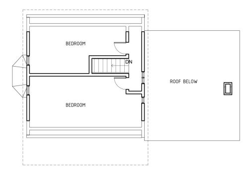
Figure 8 Cottage existing second floor plan
