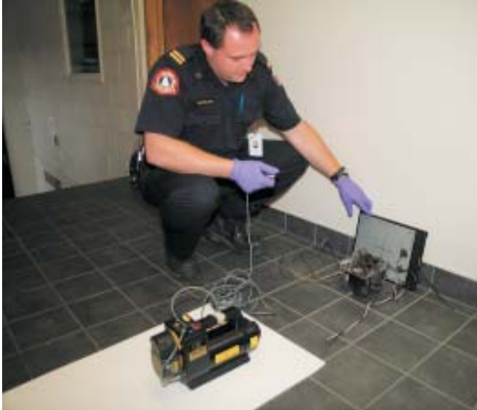
PORTABLE X-RAY – Investigator Wayne Chapdelaine uses a portable X-ray machine to look at an electrical component damaged in a recent fire. At right is the image the X-ray produced of the electrical wiring inside.
