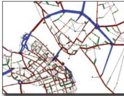
This image shows a portion of the roadway network from the QRS II Traffic Model. The thick blue bars indicate roads with high traffic volumes.
