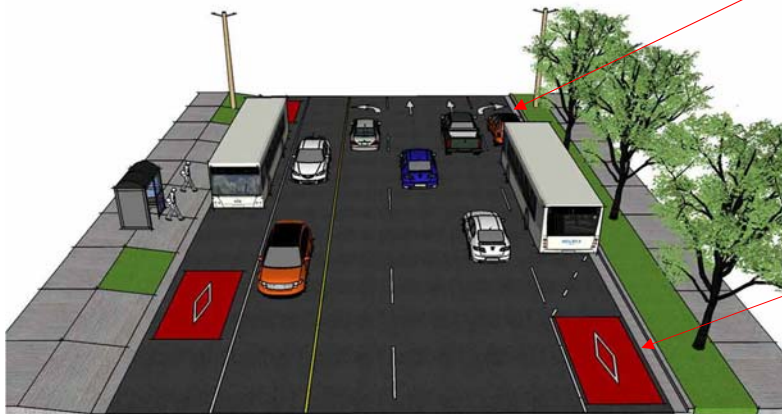
Diamond pavement markings are commonly used to identify curbside bus lanes
