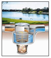
Figure 3: Typical Storm Water Treatment Unit
