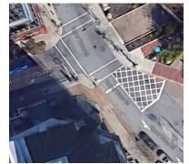
A painted intersection box is an area at or near a signalized intersection
