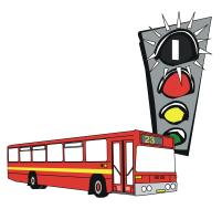
priority signal is activated a few seconds before the green light indication, but while the signal is still red for other traffic. Transit buses in adjacent traffic lanes may proceed into the intersection while the transit priority signal is on, allowing them to get a 'jump' on the rest of the traffic waiting for the green signal.
