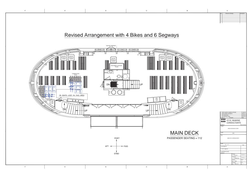
Revised Arrangement with 4 Bikes and 6 Segways 2 Bikes with Child Trailers MACHINERY EXHAUST TRUNK E.Y.E. MARINE CONSULTANTS MAIN DECK PASSENGER SEATING = 112 PORT STBD
