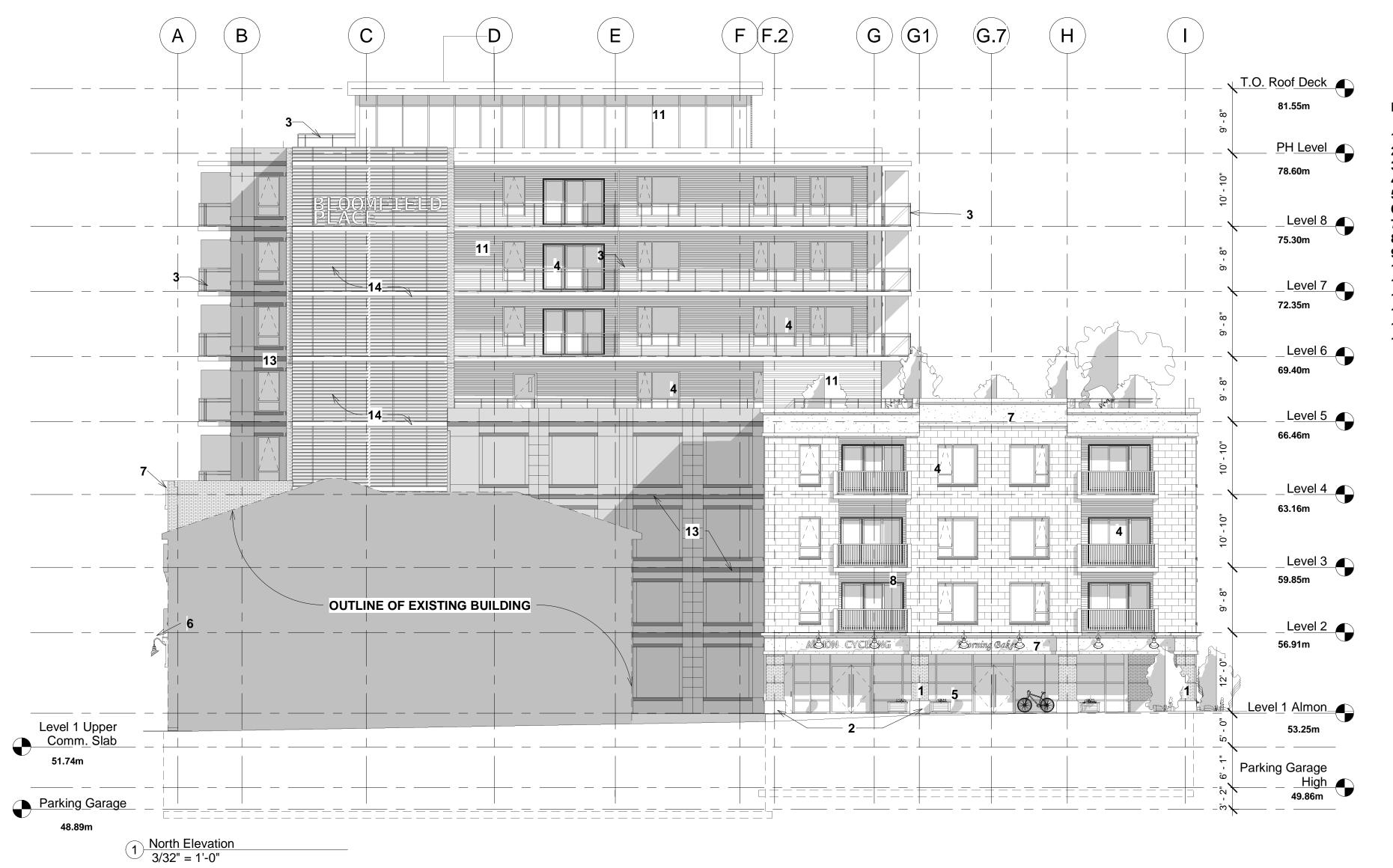
LEGEND: 1 - PRECAST PANELS OR MASONRY BRICK - TYPE 1 2 - STONE BASE 3 - 42" H. ALUMINUM/GLASS RAILING 4 - VINYL WINDOW/DOOR 5 - ALUMINUM GLAZING SYSTEM 6 - EXTERIOR LIGHTING FIXTURE 7 - STUCCO BAND 8 - MASONRY BRICK - TYPE 2 9 - FIBER CEMENT SIDING 10-42" H. METAL RAILING 11- FIBER CEMENT PANELS 12- PLANTER 13- PRECAST PANELS OR MASONRY BRICK - TYPE 3 **14- NON-COMBUSTIBLE SCREEN** 16- GLASS BLOCK (90 Min. Fire Rated)
