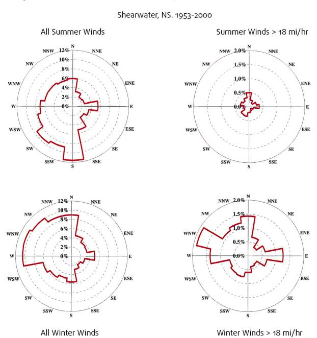
It should be noted that the building's stepped massing nature should significantly reduce wind speed in the direct vicinity of the sidewalks. Wind down gusts from the upper storeys will hit the upper raised terraces, reducing the wind speed significantly at the sidewalk but causing slightly more turbulence. In addition, canopies have been added to the commercial base, again adding a second level of wind and weather protection.
