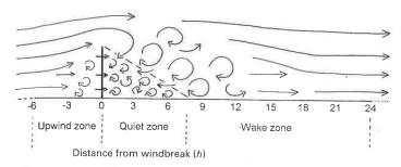
Fig. 6.4. Zones with altered airflow caused by a windbreak. Vertical dimension is magnified for illustration. Vertical line indicates windbreak; h = height of windbreak. Large eddies = strong turbulence. Uninterrupted airflow in the open is to the left of the upwind zone, and to the right of the wake zone. Widths of zones are approximate. Based on several sources.
