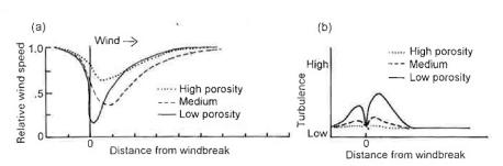
Fig. 6.5. Effect of windbreak porosity on streamline and turbulent airflows. (a) Streamline airflow based on treebelts of different foliage densities; wind measurements at 1.4 m height. From Heisler & DeWalle (1988) with permission of Elsevier Science Publishers. (b) Generalized expected turbulence pattern based on Robinette (1972), Rosenberg et al. (1983), Heisler & DeWalle (1988), McNaughton (1988).
