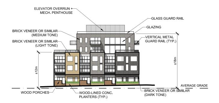
1 EAST ELEVATION A03 SCALE: 1" = 30'=0"
