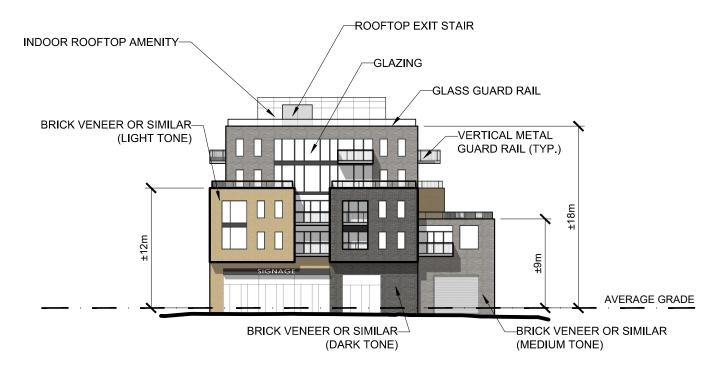
2 WEST ELEVATION A03 SCALE: 1" = 30'=0"
