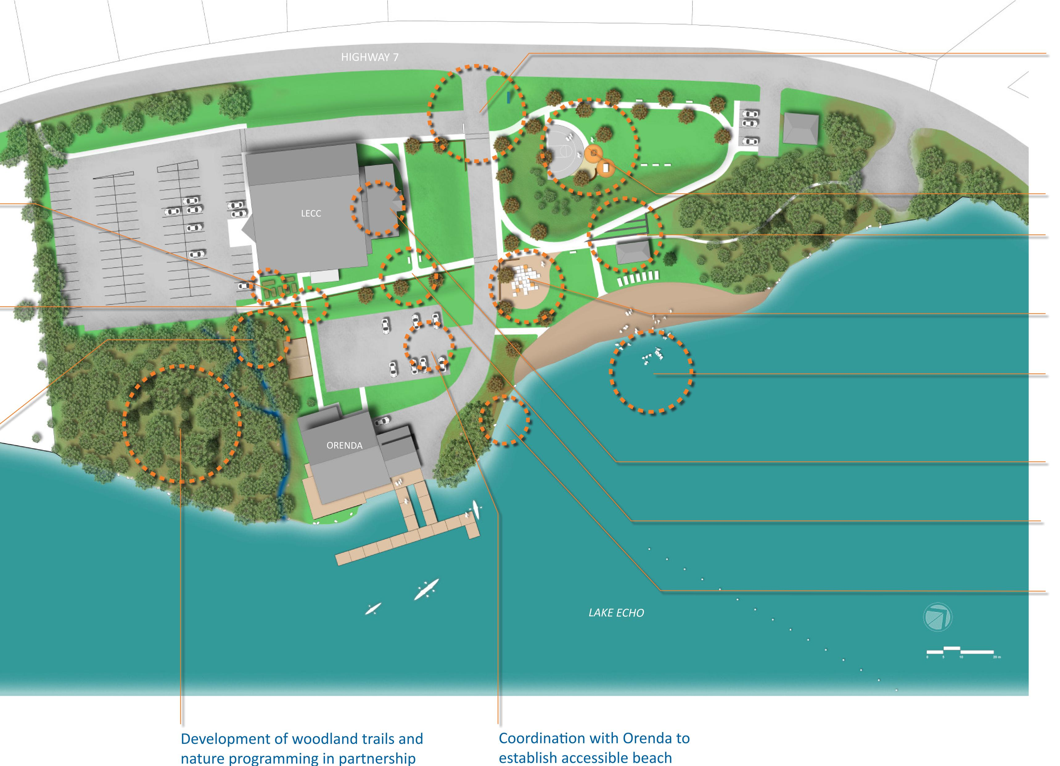
Improved circulation of vehicles by realigning the LECC driveway, thinning trees for better driveway sightlines, installing curbs, widening parking circulation driveway.
