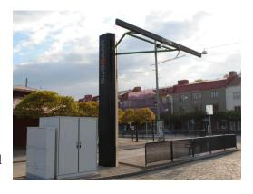
different points of the buses route. Proterra's FastFill overhead charging system, for example, can provide a full charge to an electric bus in 10 minutes (Proterra, 2013b) (Groszko, 2013).
