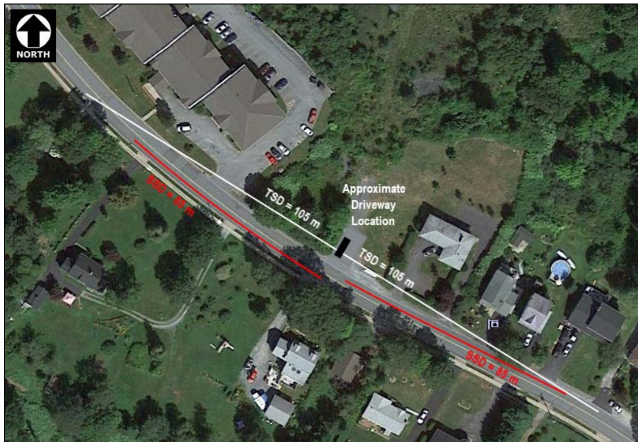
Figure 3: Approximate stopping and turning sight distance at the proposed driveway location
