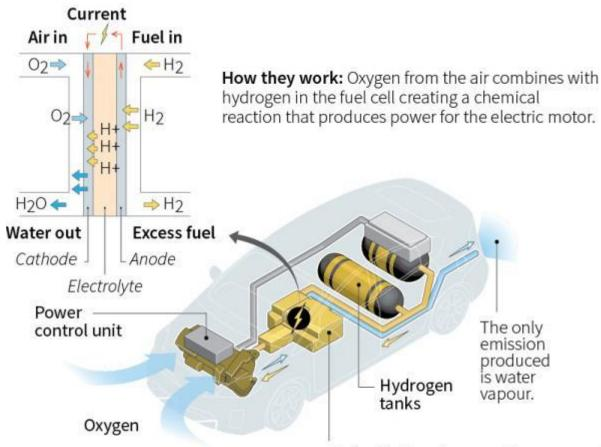
Fuel cell - Requires a continuous supply of fuel and oxygen to sustain the reaction.
