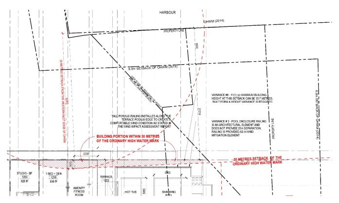
Image 6: This image shows portion of the north-east building face on level 12 that is within 30 metres of OHWM and over the required 33.7 metres of building height limit
