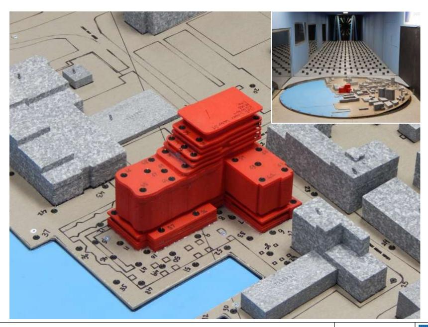
Wind Tunnel Study Model **Proposed Configuration**
