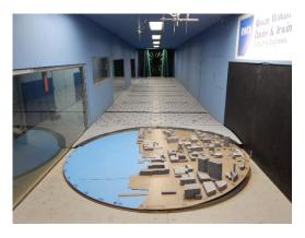
Image 1a: Wind tunnel model of the existing site and surroundings in 2015
