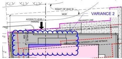
Image 2: shows the mid-rise portion of the building along Bishop's Landing encroaching the 5.5 metres setback line from the interior lot line
