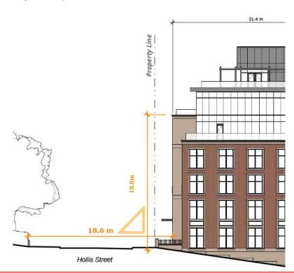
Figure 2: Effective Right of Way to streetwall provides nearly a 1:1 ratio
