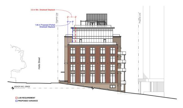
Figure 11: South elevation illustrating requested variance of upper streetwall stepback on Hollis Street to 1.85m
