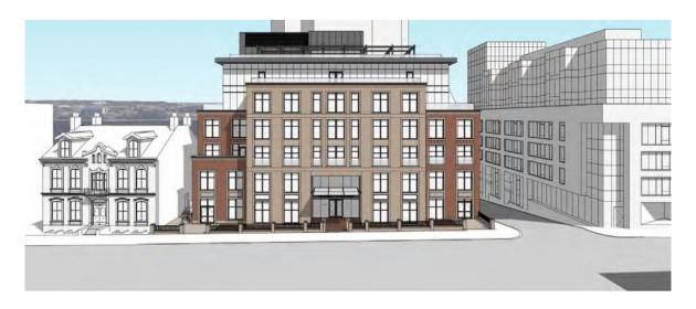
Figure 12: Hollis Street frontage illustrating the recessed "wing" streetwalls ceding prominence to the central streetwall, as well as the minimal design of the façade above, to avoid distraction from the heritage-inspired design of the streetwalls.
