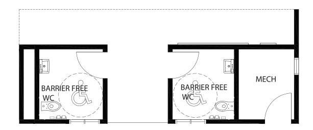
FIGURE 47. Permanent mini-washroom 25–35 m² total gross floor area \$2,500 to \$3,500 per m² \$122,500/facility per above plan
