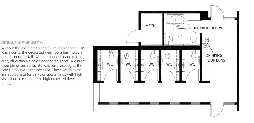
FIGURE 46. Dedicated washroom  $50-60 \text{ m}^2$  total gross floor area \$3,000 to \$4,000 per m<sup>2</sup> \$240,000/facility per above plan
