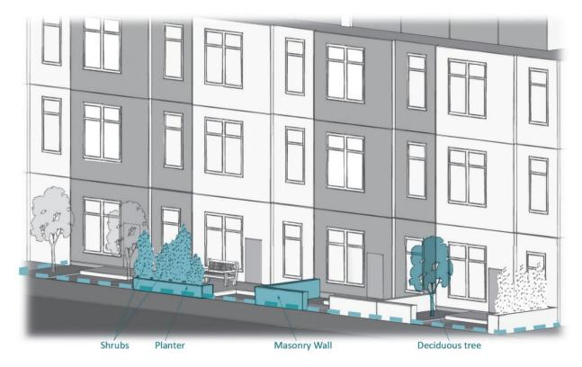
(d) masonry walls ranging in height from 0.25 to 1.0 metres.
