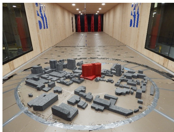
Diagram A1-2b: Photo of modelled buildings in a boundary-layer wind tunnel
