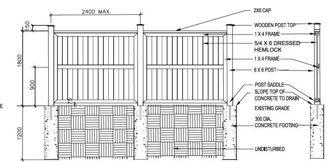
3. ALL FASTENERS TO BE GALVANIZED OR RESISTANT TO CORROSION.
