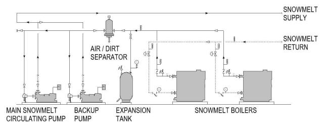
Snowmelt system schematic using dedicated boilers
