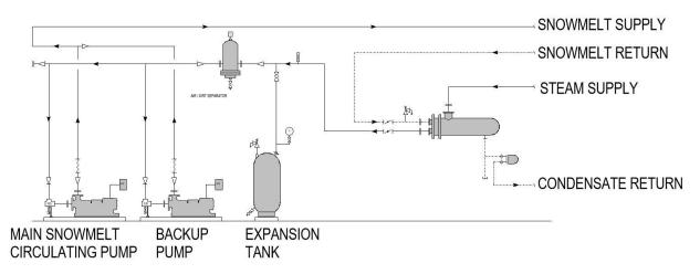
Snowmelt system schematic using steam from MSVU Heating Plant.
