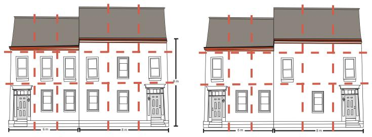
Front façades showing variable appropriate widths, including three bays each, and a cornice line of less than 8m in height. Both images show windows which are taller than wide. The image on the right demonstrates one possible fenestration pattern which satisfies only the minimum requirement of one window within each bay and storey.
