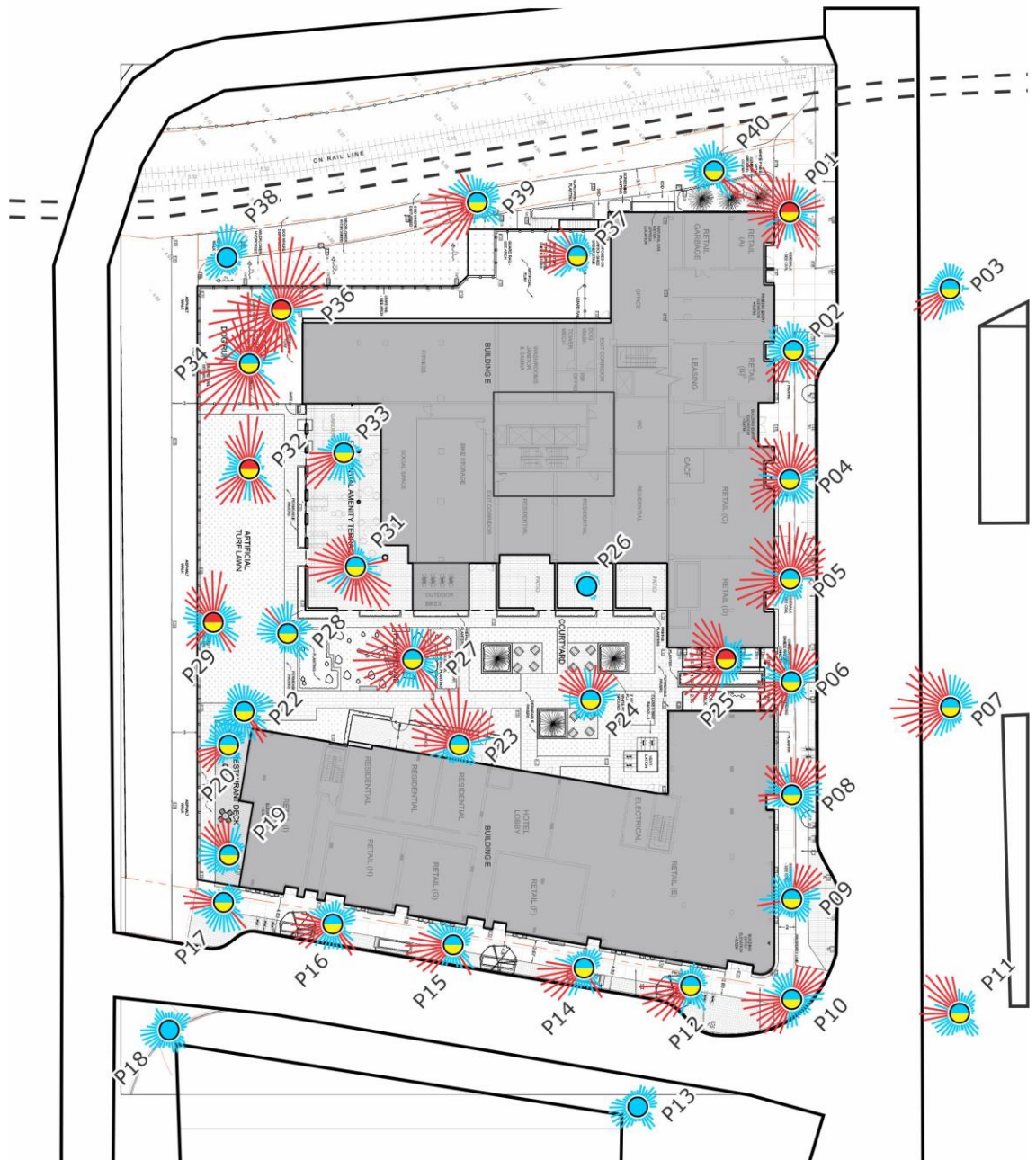
Figure 6: Wind Tunnel Results (Summer) – Parking Level 0 and Level 1 Plan Proposed Site Conditions (results shown without treatments applied)
