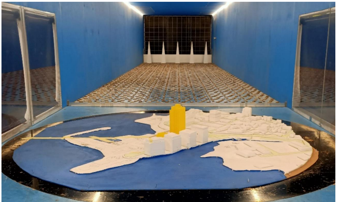
Figure 1i: Photograph of the Wind Tunnel Model – Proposed Scenario (view from the east)
