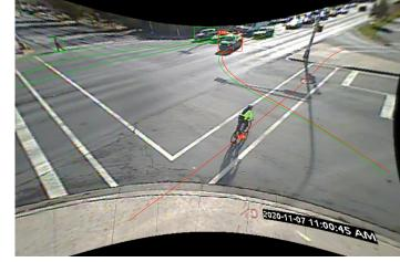
Cyclist North Left-Hook: T2 = 2.5s, vehicle speed: 21 km/h, cyclist speed: 25 km/h
