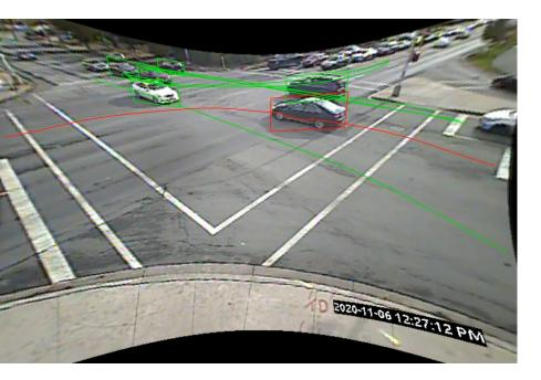
East-left vs West-through: PET = 1.6s, vehicle speed: 56 km/h
