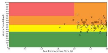
The LTAP conflict data, for example South-left vs Norththrough (above) and North-Left vs South-through (below), shows several conflicts occurring with through vehicle speeds exceeding the posted speed limit of 50 km/h (up to ~75 km/h).
