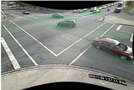
West-left vs East-through: PET = 2s, vehicle speed: 43 km/h
