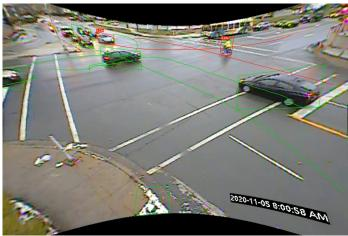
Cyclist East Left-Hook: 12 T2 = 2.5s, vehicle speed: 20 km/h, cyclist speed: 18 km/h
