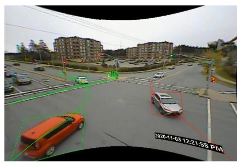
West-Left vs East-Through: PET = 1.5s, vehicle speed = 65 km/h
