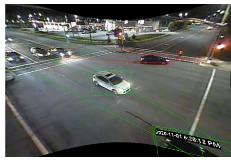
Pedestrian North Left-Hook: T2 = 2.4s, vehicle speed = 17 km/h
