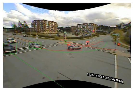
Pedestrian West Left-Hook: T2 = 2.2s, vehicle speed = 11 km/h
