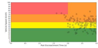
East-left vs West-through (above) and West-Left vs East-through (below) conflict data shows several conflicts occurring with through vehicle speeds exceeding the 60 km/h posted speed limit (up to 75 km/h).
