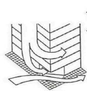
A tall building concentrates wind at its base, particularly at the corners where the downwash is accelerated into horizontal motion.
