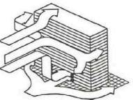
Openings through a building at the base induce high velocities due to pressure differential from the front to the back.
