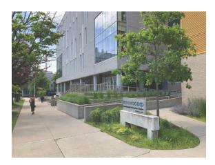
Figure 4.3.3: Appropriate Institutional Setback. Approximately 4.0 m from the streetline and comprised of vegetation, an extended sidewalk, seating, and entrances.
