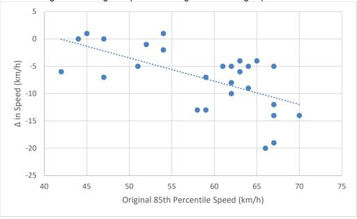
Figure 1: Change in speed following traffic calming implementation
