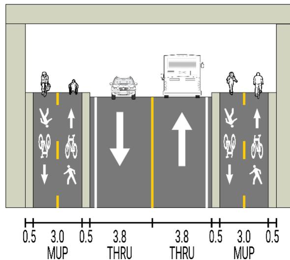
Figure 10 - Near-term cross section at the Highway 102 underpass for multi-use pathways on both sides alternative
