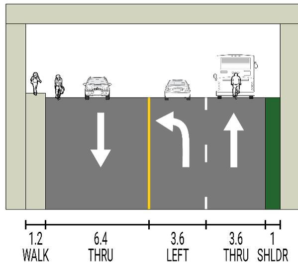
Figure 6 - Cross section of existing underpass (looking west)
