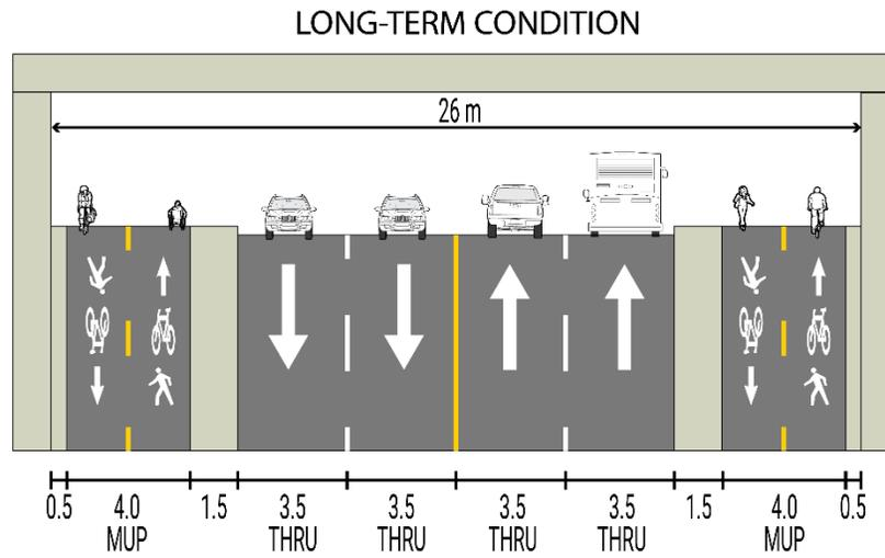
Figure 15 – Recommended long-term underpass cross section
