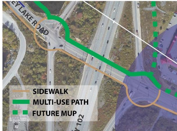
Figure 11 - Active transportation facilities associated with the multi-use pathway on one side alternative
