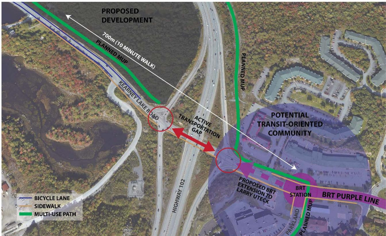
Figure 7 - Existing active transportation connectivity through the interchange
