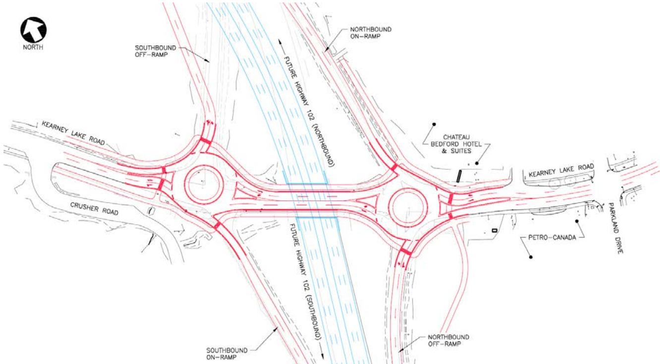
Figure 14 - Preliminary layout of long-term design
