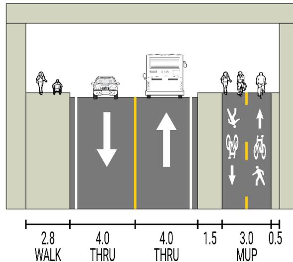
Figure 12 - Near-term cross section at the Highway 102 underpass for multi-use pathway on one side alternative
