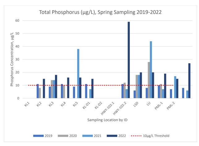
Figure 1: Total Phosphorus Concentrations from the Bedford West Water Quality Monitoring Program, Spring Sampling Events, 2019-2022
