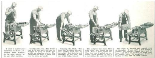
Figure 13: Explanation of how to use concrete block machines (Source: Sears, Roebuck, and Co.)
