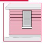
Install non-combustible siding (stucco, metal, stone, cement fibre board).
