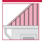
Install Class A fire-resistant roof covering (e.g., cement fibre, metal or asphalt shingles).
