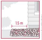
[5] Install non-combustible ground surfaces within 1.5 m of the house (mineral soil, rock, concrete or stone).
