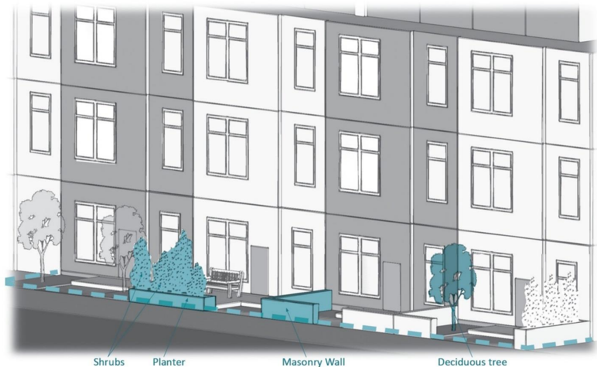
Diagram 8: Methods for privacy for grade-related units, as per Section 119
