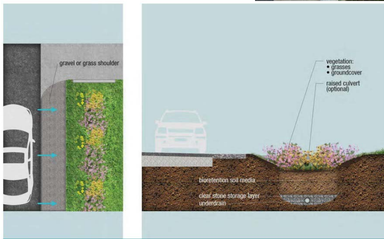
Figure 2.2.5: Bioswale plan view (left) and cross-section (right)
