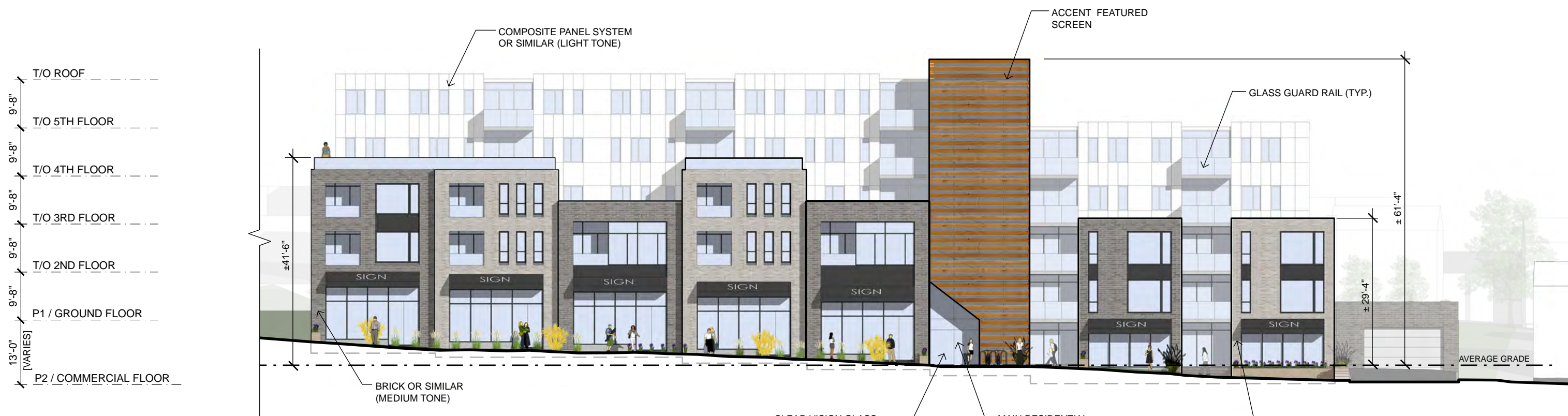
2 BUILDING A - WEST ELEVATION SCALE: 1" = 20'-0"
