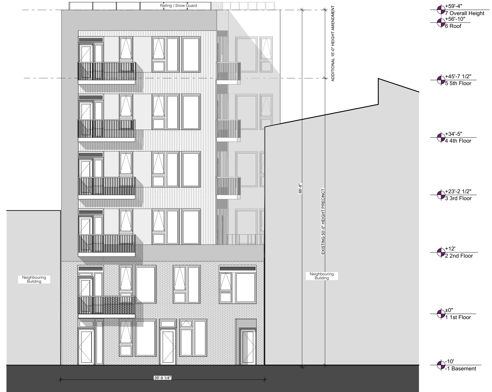
East Elevation - From Rear of Lot
