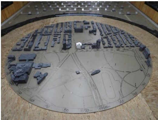
Image 2A: Wind tunnel study model - Existing configuration
