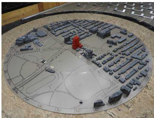
Image 2B: Wind tunnel study model - Proposed configuration
