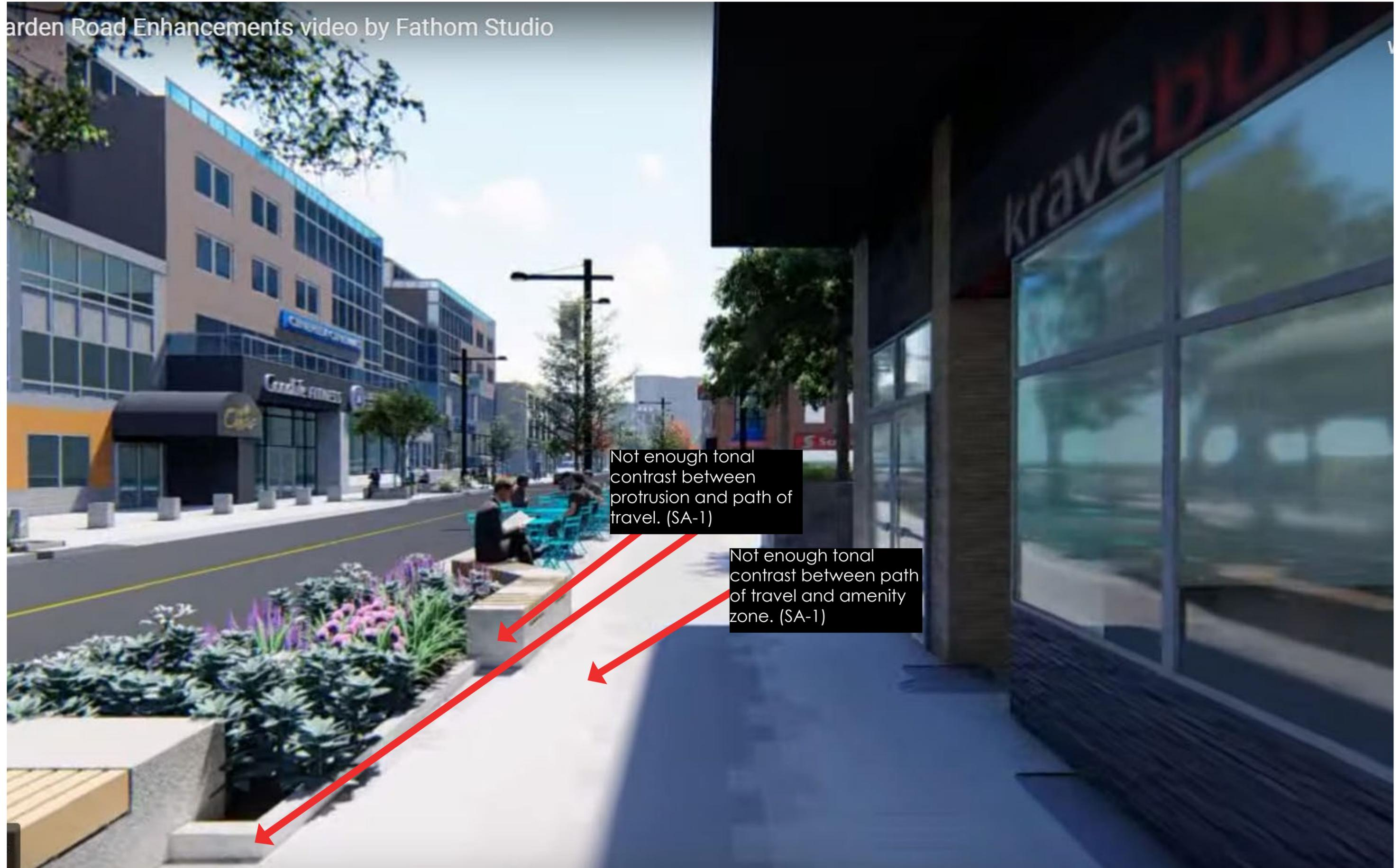
Not enough tonal contrast between protrusion and path of travel. (SA-1)
