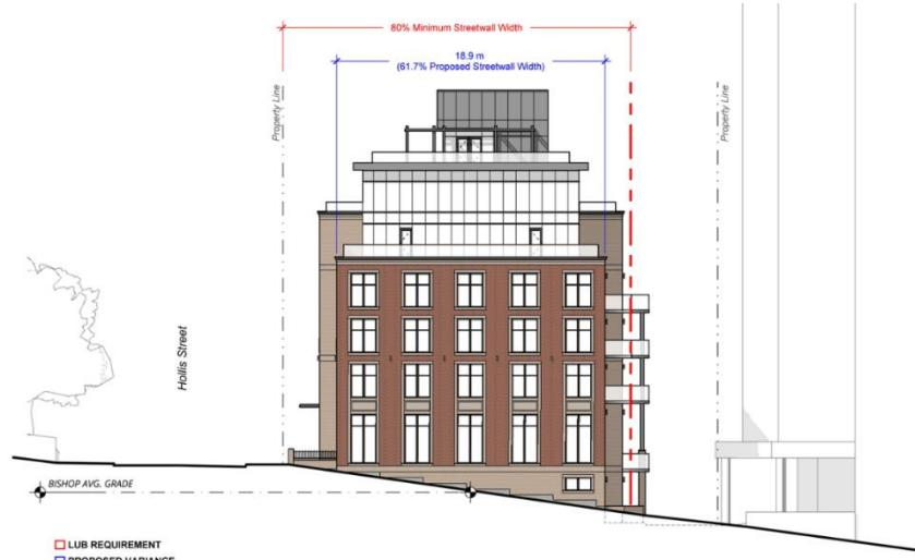
Figure 9: Illustration of requested streetwall coverage variance
