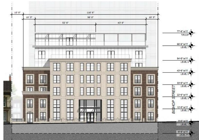
**Image 3 – West Elevation of the Proposed Development – View from Hollis St.**
