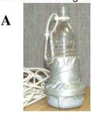
Please keep your Secchi disk to use in following years. With time, some rope material will stretch. Each year check that the metre markings on the collection bottle rope and the tenths of a metre markings on the Secchi disk rope are still accurate.
