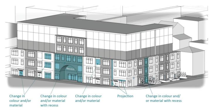
Diagram 9: Methods for streetwall articulation, as per Section 121
