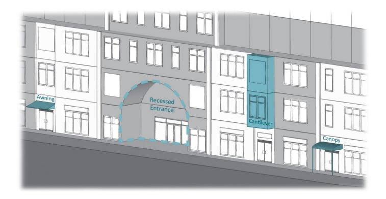
Diagram 11: Methods of weather protection, as per Section 130
