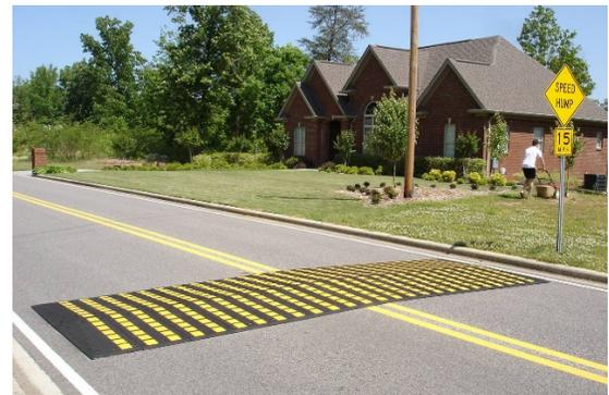
Sample of a speed hump used for traffic calming
