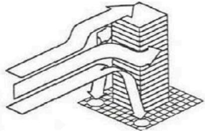
A tall building concentrates wind at its base, particularly at the corners where the downwash is accelerated into horizontal motion.
