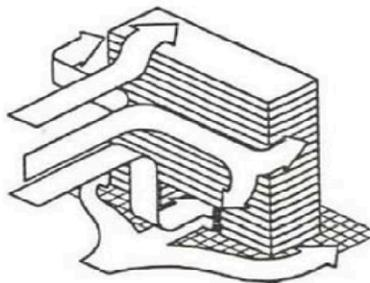
Openings through a building at the base induce high velocities due to pressure differential from the front to the back.
