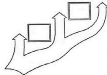
Adjacent building placement can cause a compression of the mean streamlines, resulting in horizontally accelerated flows at ground level.
