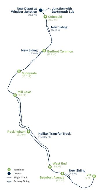
Figure 21: Commuter Rail Operating Schematic
