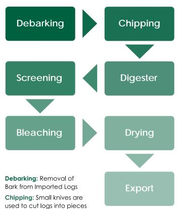
Digester: Addition of Sodium Hydroxide and Sodium Sulfide. This process "cooks" the material
