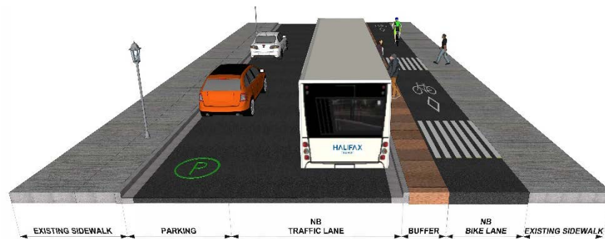
HOLLIS STREET (LOOKING SOUTH) AND LOWER WATER STREET (LOOKING NORTH), TYPICAL TRANSIT STOP
