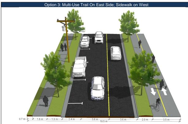
Figure 4: Cross-section of Option 3
