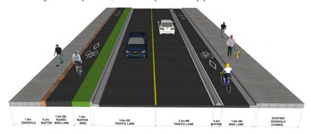
Figure 4-4: Concept Design - Option A (Typical)
