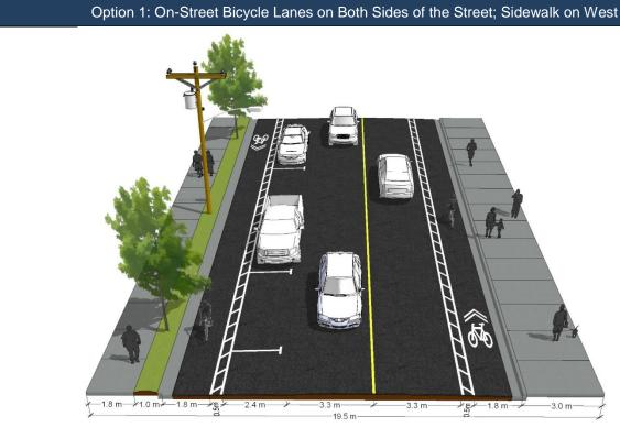
Figure 2: Cross-section of Option 1
